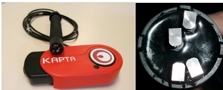
Figure 2: GSM communication module (left) and Kapta™ 3000 OT3 (right)
