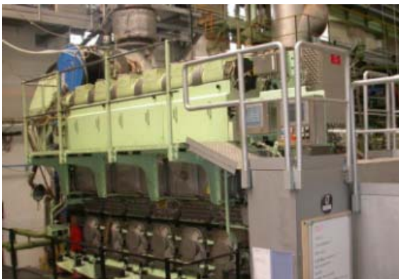
Figure 5.2b. The 4-stroke test engine with the SCR unit (left) and the temperature study on that SCR engine (right)
