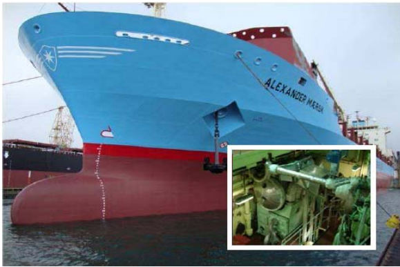
Figure 5.2a. The EGR installed on-board Alexander Maersk (left) and the High Pressure Boiler installed on the 4T50ME-X 2-stroke test-bed engine (right)
