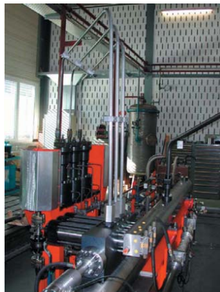
Figure 8.1b. The Common Rail (CR) test rig for 2-stroke engine application
