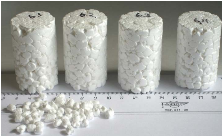
Figure 2: Expanded PLA/wood-fibre composite particle foams.
