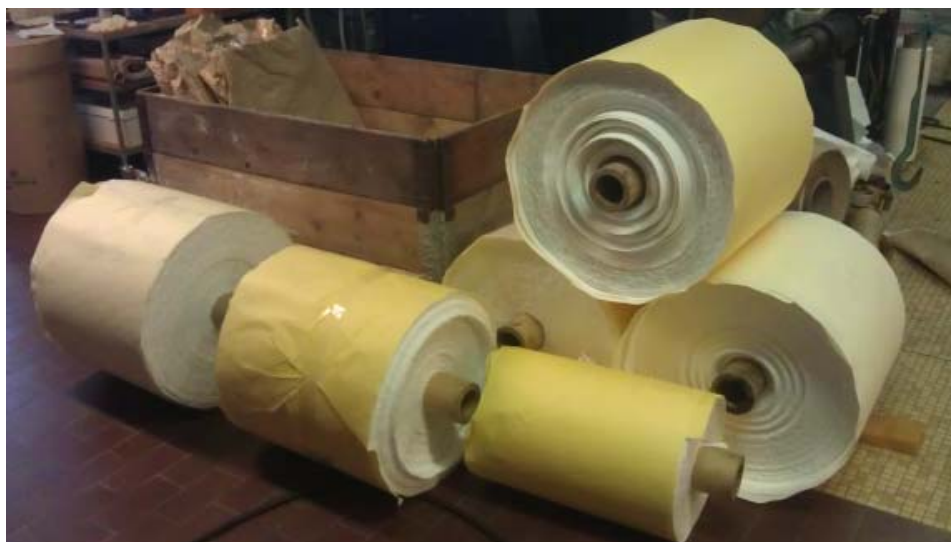
Figure 5: Rolls of wet-mixed wood-fibres and PLA. The sheet material was produced in pilot-scale on a paper machine.
