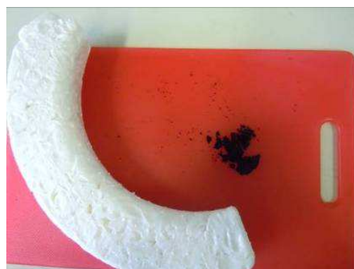
Figure 13 - The porthole spacer before and after disintegration in home composting conditions
