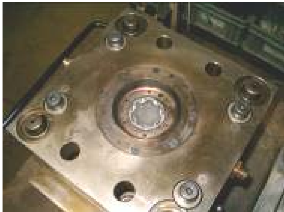
Injection mould after production of 10000 pieces
