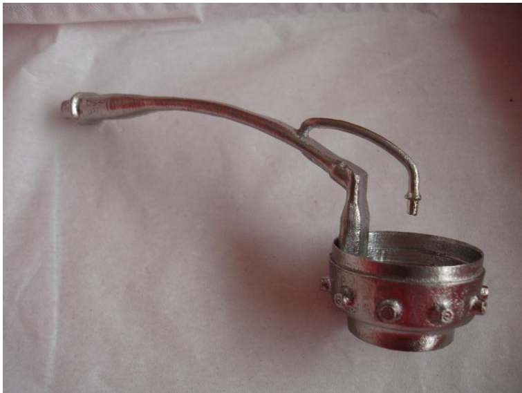
Figure 28 Part detached and after a surface finishing.
