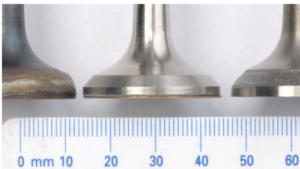
Figure 24 To the left is a conventionally produced clad (non-laser) to the right is a laser deposited valve and the centre is a machined OSVAT valve.
