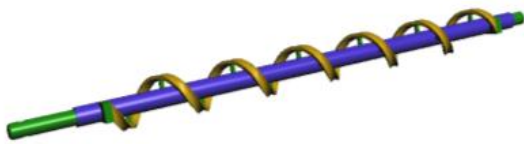
Figure 14 The proposed new powder stirrer for the powder feeder for the powder bed process.
