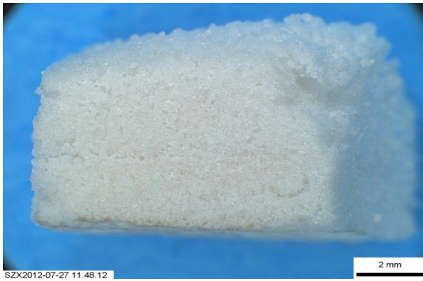
Figure 12 Alumina block produced using laser powder bed technology.
