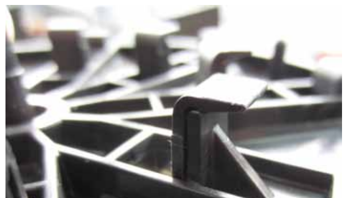
A green house fan: This product required excellent impact resistance, light weight and a more resilient, secure snap-fixing. Successfully delivered with a PET/ PP combination
