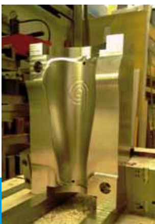
A football shin guard tool in production. The SRP materials give a lightweight, stiff, impact resistance compression moulded product.
