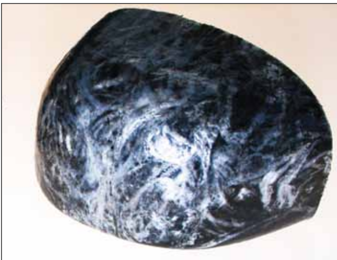
Safety shoe cap manufactured by inductively heated HDPE/PP sheets
