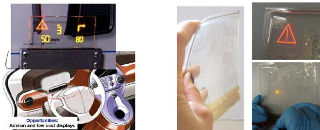
Figure 3. Emissive head-up displays developed in NaPANIL. In addition to glass-based display, also a conformal demonstrator was realised.
