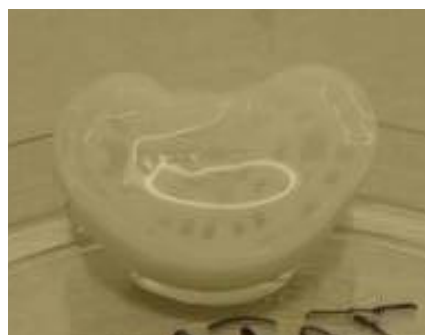
Custom-made and gel-loaded IVD scaffold
