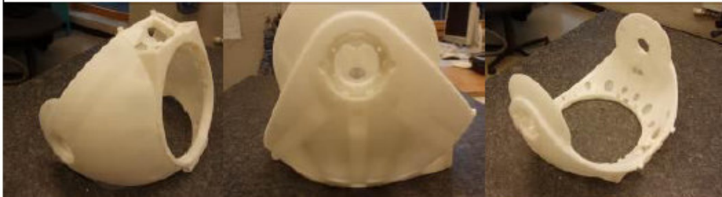
Part showing good resolution/roundness of small bores and surface quality; weight: ~273 g
