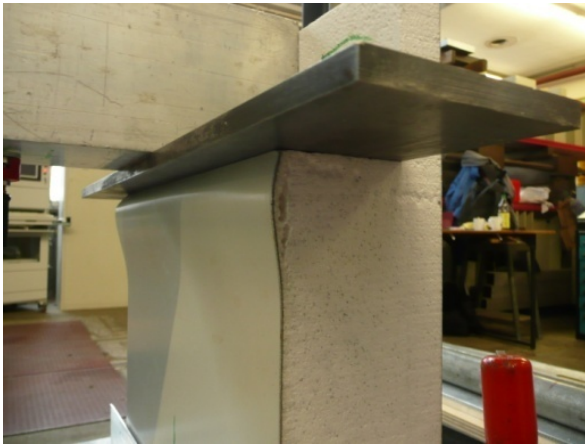
Fig. 3.5: Crippling of the load application area
