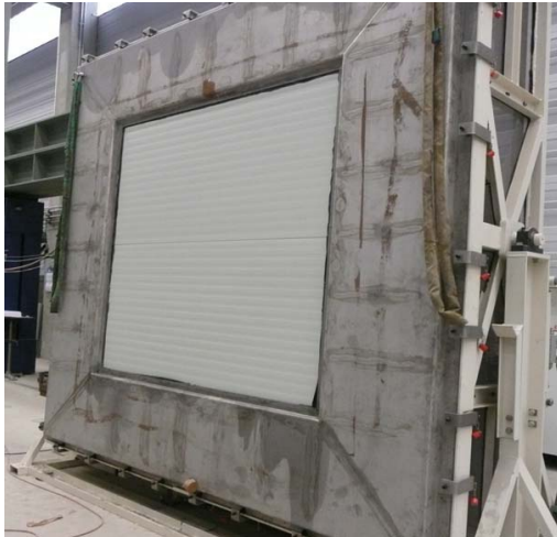
Fig. 1.1: Tests on panel assembly to measure joint air tightness
