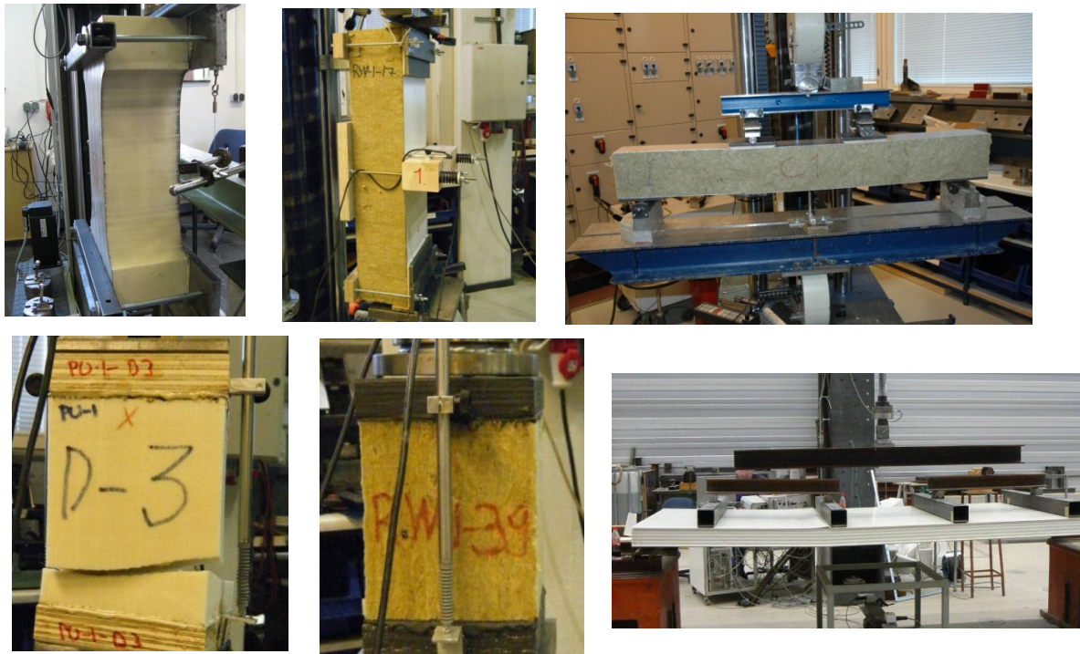
Fig. 4.1: Bone-shaped and rectangular wrinkling test specimens, shear test specimen, cross-panel tensile and compression test specimens and full-scale specimens made of PU- and ESP-foam cored and stone-wool cored sandwich panels were used in the durability studies.
