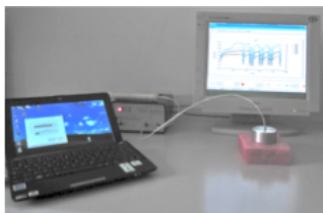
Figure 4 : Experimental setup for freeze-drying bacteria quality test. Bacteria are kept under the sampler at the right. The electronic unit in the background captures the headspace and delivers to the internal sensor array.
