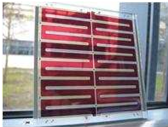
Figure 5.1. A 10x10 cm 2 current-collecting double glass-substrate sandwich devices from ECN /Fraunhofer ISE.
