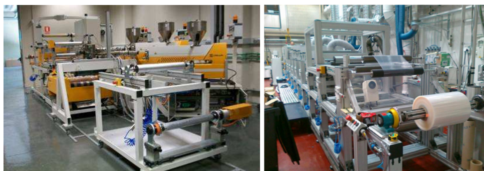
Figure 7. Pictures of the pilot plant equipments used in the project (coextruder line and coating one).
