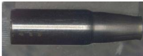
Figure WP1.8: EMPT joined sample (Courtesy A. Cambriani, JRC-ITU)
