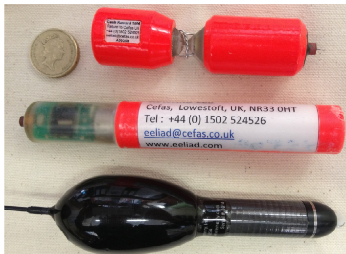
Figure 1.1.2. External tag types used on eels. Top two examples are Cefas flotsam tags (or 'e-DST'), while the lower tag is a Microwave Telemetry PSAT.
