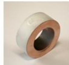
Airbrush/Cu (sand blasted)/ZrO 2 /Silicone/ 200° C/1h/Air/ ca. 200µm
