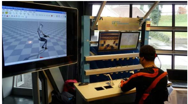
Ergonomics evaluation: automatic physical and cognitive load analysis, full body motion capture
