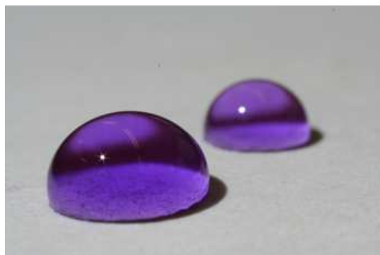
Figure 33: Droplets of water at the surface of coated and grafted paper after 5 minutes of exposure. Source D. Guérin, Centre Technique du Papier.
