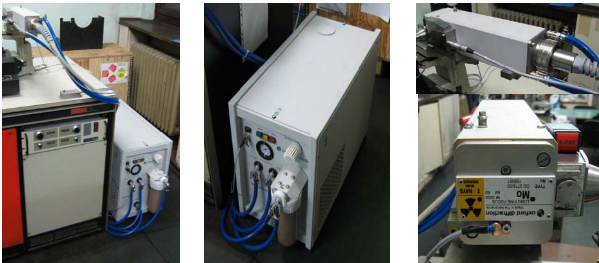
Powder diffractometer upgraded (left), water chiller unit for fine focus X-ray tube cooling (middle), and X-ray tube (with Mo X-ray tube) shield housing and shutter control box (right).
