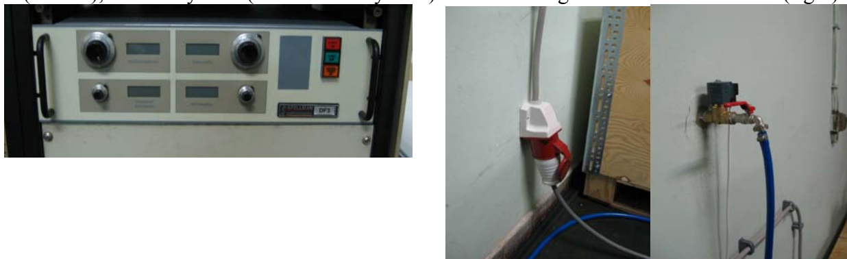
X-ray generator Spellman DF60N3 (3 kW) (left) and the renewed electrical and water connections for the instrument (right).
