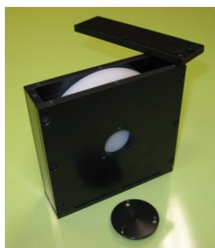
Fig. 5.4 Responsivity phantom (PTB). For characterization of the phantoms see [H. Wabnitz et al., Proc. SPIE 7896 (2011), 789602].
