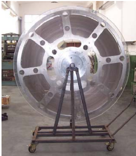
Figure 2: Picture of a 1.7 km conductor on its spool after completion of the production phase 5
