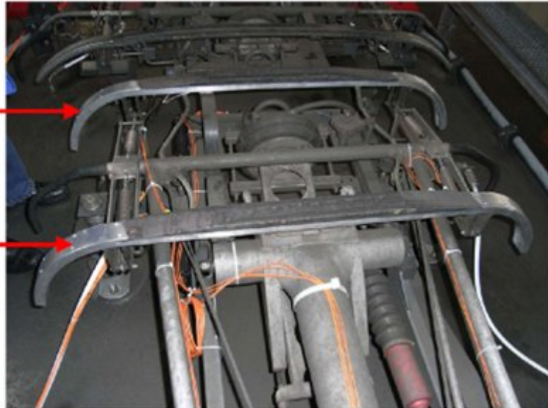
Figure 1.2.11: Smart Current Collectors installed in ÖBB RH1216-143 dc pantograph
