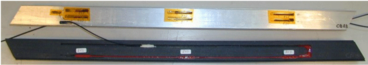
Figure 1.2.8: Carbon bar and Al profile with attached sensors before assembly. Grooves in carbon with old design. Grooves are refilled with silicon to save the sensors in the assembly process.
