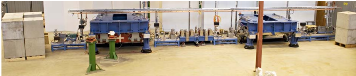
Figure 6: The optical klystron (modulator undulator- chicane - radiator undulator) at MAX-lab. The electron beam enters from the right.
