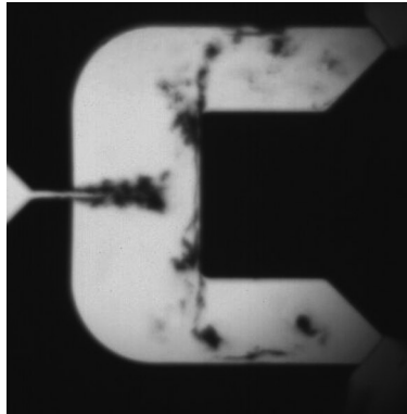
WP_2_BOSCH_Figure_1: Cavitation experiment – throttle flow combined with stagnation point flow.
