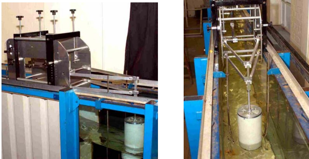
Fig. 4: Laboratory model for validation of the PTO simulation in a narrow wave tank
