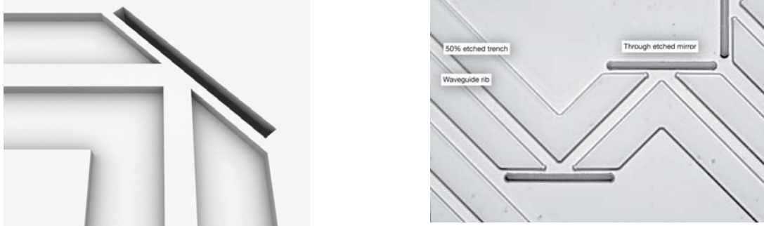
Fig. 11: Basic design of a waveguide mirror (left) and microscope image of a waveguide mirror fabricated in 4 \mu\text{m} SOI
