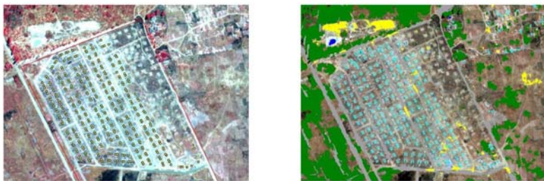
Results of the visual detection (left, 346 buildings) and the semi-automated extraction (right, 393 buildings).
