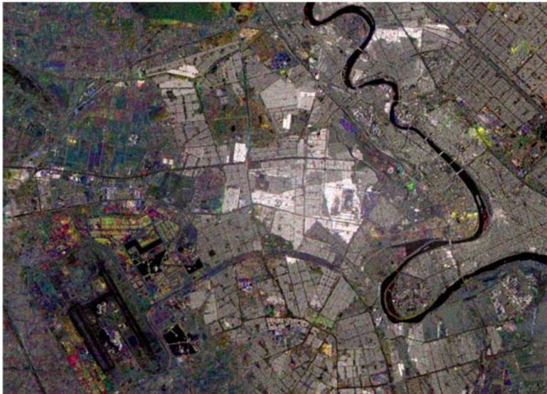
Multi-temporal Radarsat image of the Baghdad area from 23 April 2003 (blue), 17 July 2005 (yellow) and 2 April 2007 (red). Colours indicate change.
