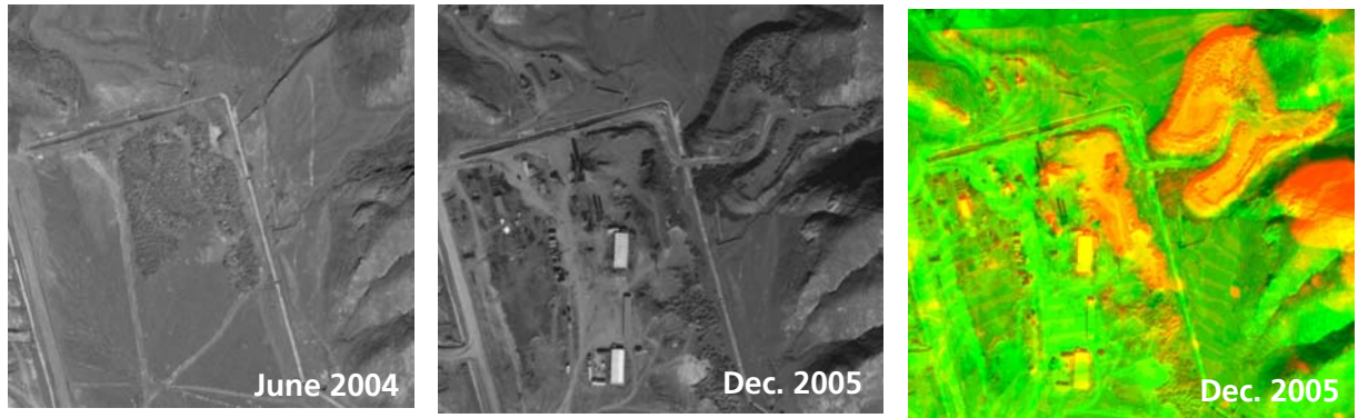
Figure a, b, c: Two images of different dates and combination of Orthoimage (green) and difference of two digital surface models (red). Maximum height difference is 10 m.
