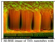
SE/BSE image of TiO<sub>2</sub> nanotubes with one W marker layer.
