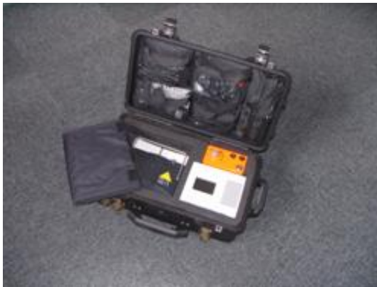
Figure 2 : Transportable terminal and its foldable solar charger
