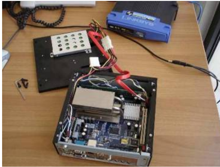
Figure 7: Remote control hardware solution
