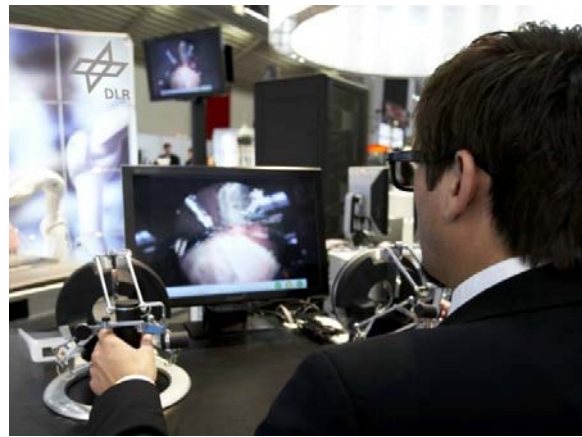
Fig. 3 The MIRS remote master station with two haptic devices and a user testing the force feedback with a beating heart
