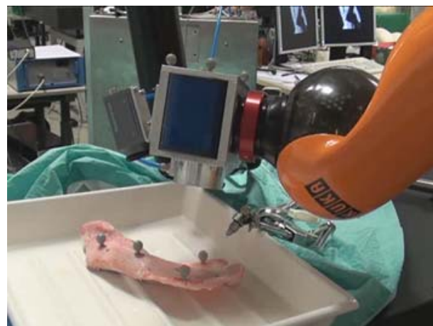
Setup for robot-assisted laser bone ablation.
