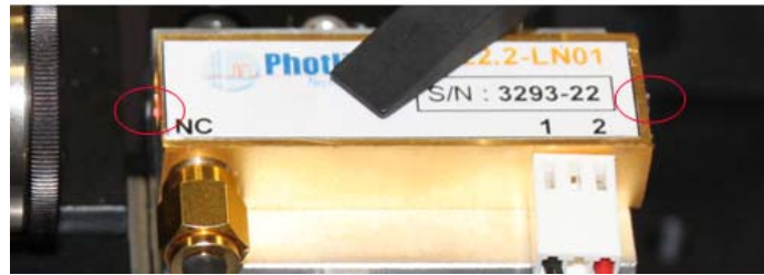
Fig. 4.10: Close-up of the modulator showing the bare guide ends – circled.
