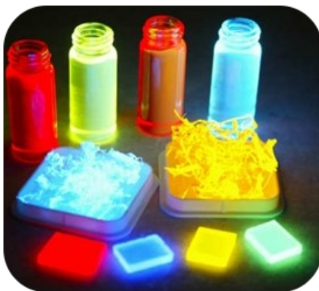
Figure 2: Photograph of conjugated polymers in liquid, powder and thin film form. Conjugated polymers and oligomers are the main active materials used in the POLYCOM project.
