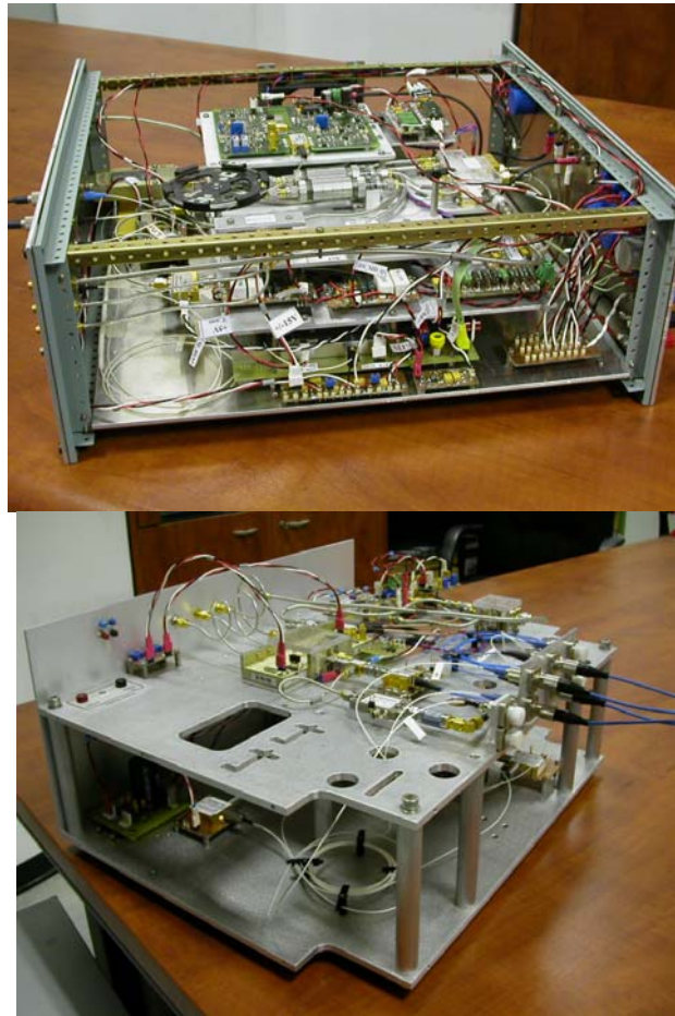
Figure 47 - Photos of the assembled 21.5 Gbaud RZ-DQPSK transmitter and receiver
