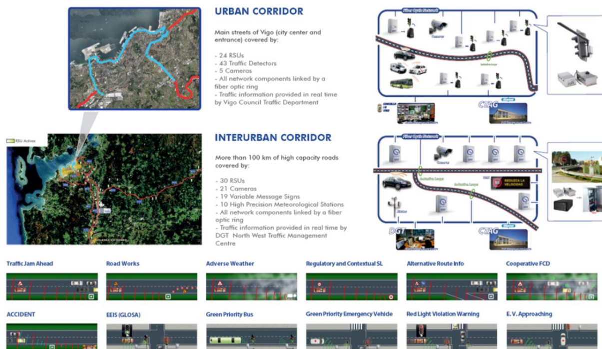
Figure 5: Available C-ITS infrastructure and services in the area of Vigo
