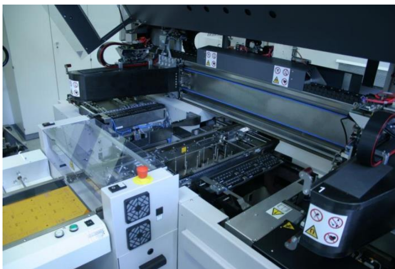
Figure 15 : Fully automated assembly equipment (SiPlace) for component mounting can be used to with SCB substrates.
