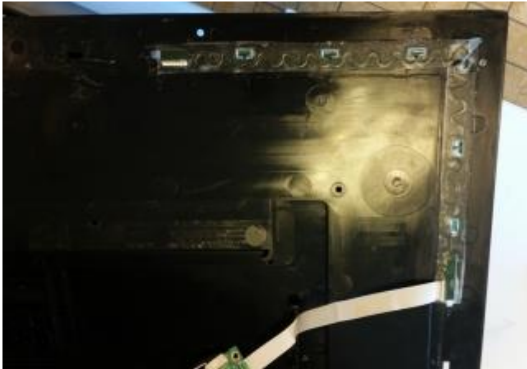
Figure 63 : Flex PCB strip bent over 90° applied to a TV back cover
