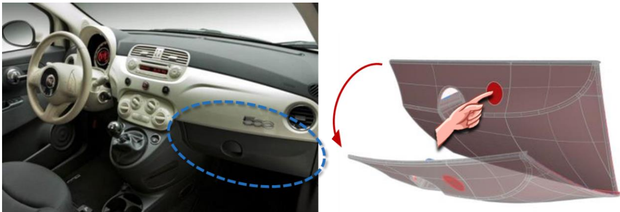
Figure 55 : FIAT 500USA glove box currently in production with manual opening (left), glove box with touch sensor and automatic opening (right)
