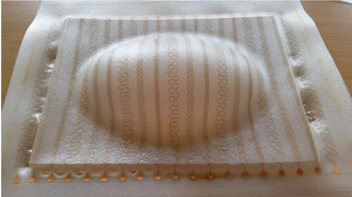
Figure 33 : Testvehicle including different variations of meanders
