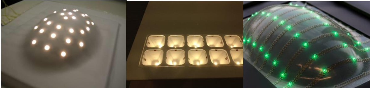
Figure 39 : Examples of testvehicles with integrated LEDs
