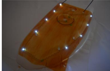
Figure 26 : SCB circuit after pre-heating and overmoulding
