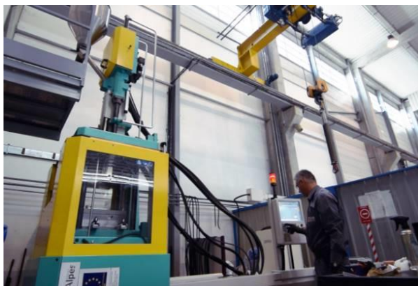
Figure 20 : Vertical injection moulding machine for overmoulding trials
