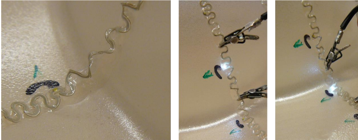
Figure 47 : Thermoformed test vehicle with components with different size, orientation and bond pad finish. Despite delamination, strain and deformation, all contacts and tracks remained intact. The two right pictures show a still working LED.
