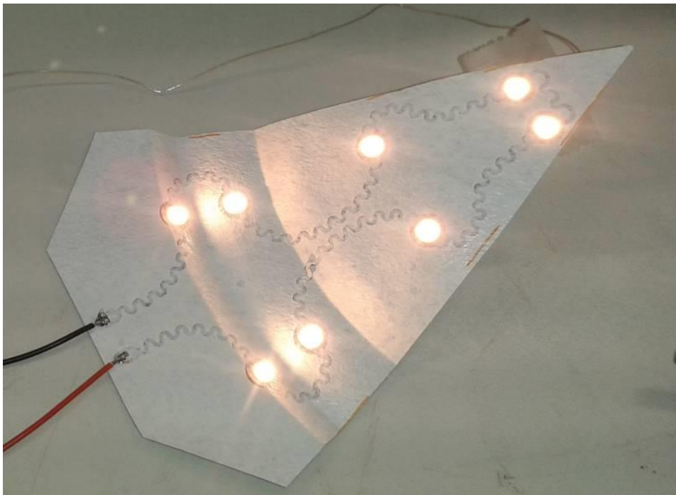
Figure 45 : Philips cakepiece design: SMI technology
