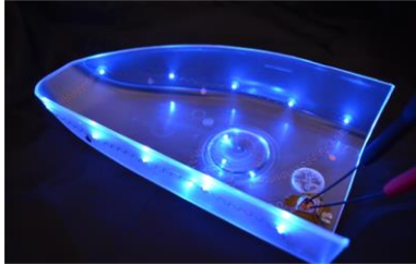
Figure 25 : SMI circuit after thermoforming and overmoulding
