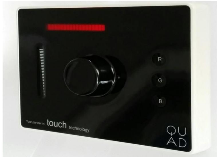
Figure 66 : Final assembled module of the Quad demonstrator.
