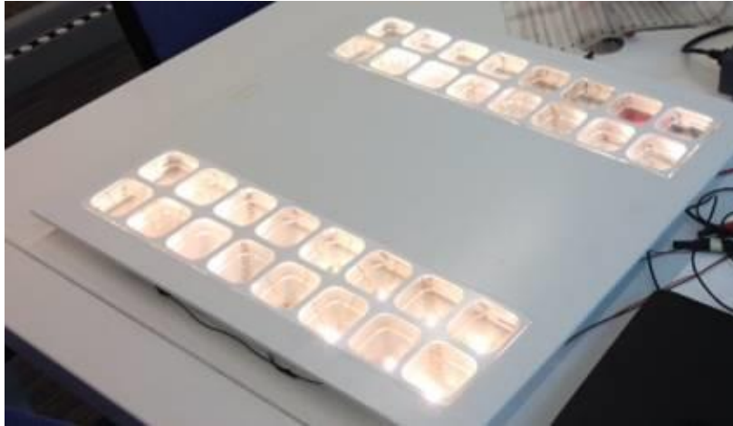
Figure 72 : Luminaire with built-in parts based on SMI technology
