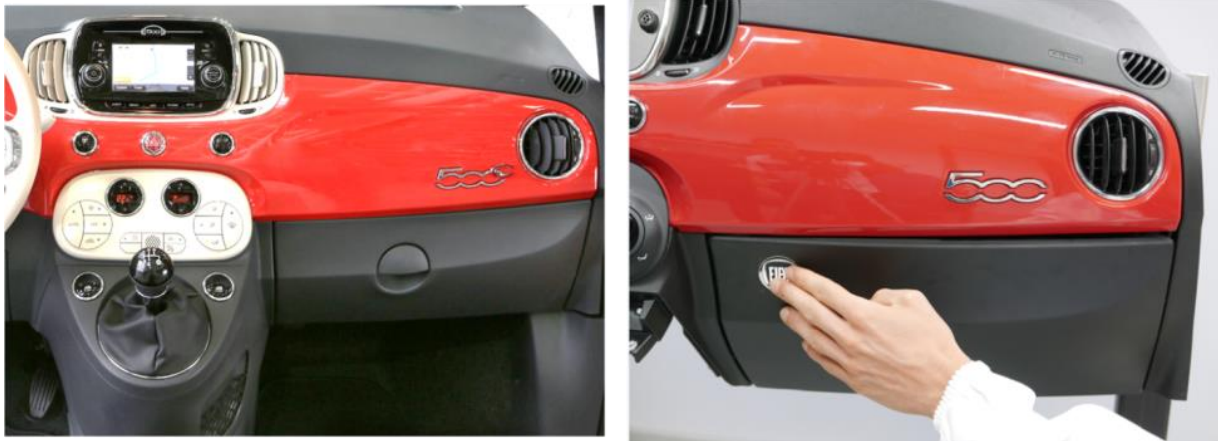
Figure 58 : FIAT 500 dashboard. On the left the standard glove box, on the right the smart glove box with embedded electronics.
