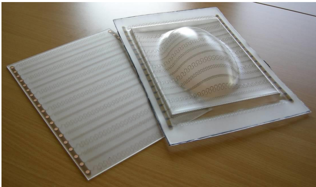
Figure 7 : Parallel meander test vehicle before and after forming.
