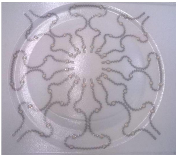
Figure 49 : Generic test vehicle for cost modelling and cost break down for the substrate technologies
