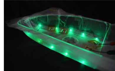
Figure 27 : SPF circuit after pre-heating and overmoulding
