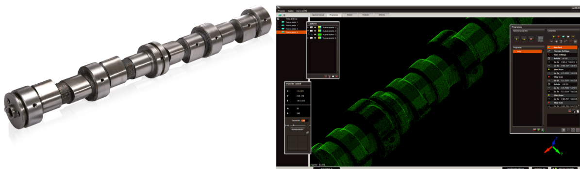
Figure 1: Physical part and pointcloud after scanning for advance processing and analysis in dimensional quality control
