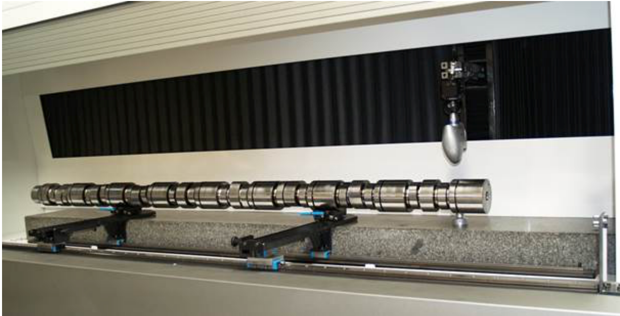
Figure 2: 3D dimensional quality control equipment used for camshaft digitalization
