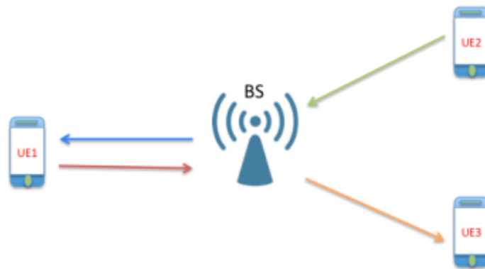
Figure 10. A LTE small cell with a full-duplex BS and co-existing full-duplex and half-duplex UEs.
