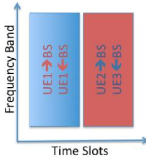
(b) User scheduling method 1 with TDMA multi-user access scheme.
