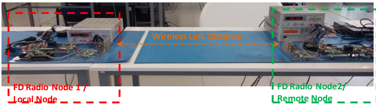
Figure 63. Picture of the evaluation setup for the dual-port antenna demonstrator.
