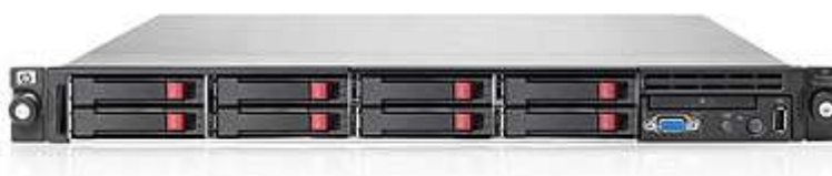
Fig. 6 - Picture of the server HP ProLiant DL360 acquired for the virtualization services
