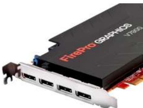
Fig. 8 - Picture of the graphic card AMD Firepro V7900 and the four display outputs
