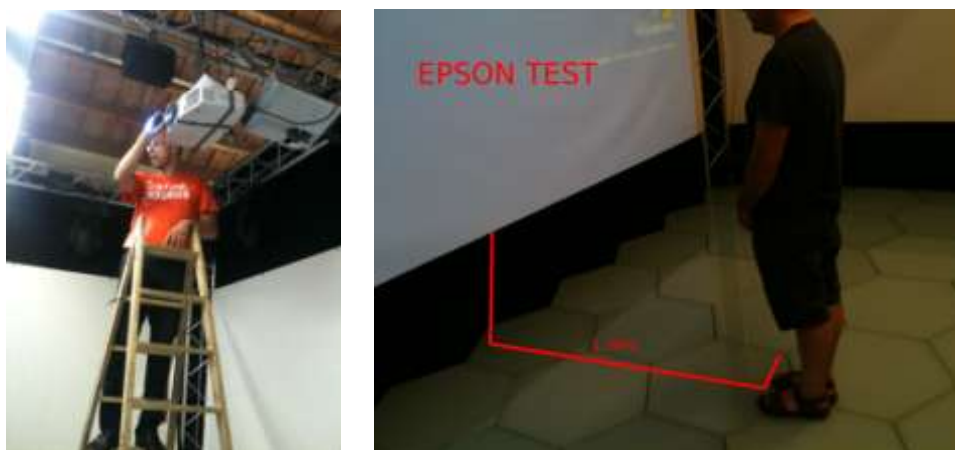
Fig. 13 - Images of the projection test in the XIM room. The left image shows the equipment mounted and the right image shows the test made to measure the maximum distance without shadows using one projector per screen.
