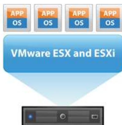
Fig. 7 - Schematic view of the VMware ESXi software that allows creating virtual machines over a unique server.
