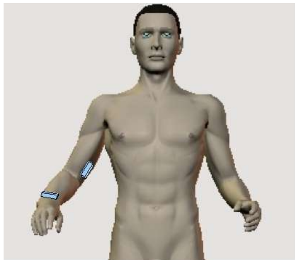
Fig. 2 - Possible inertial sensor positioning
