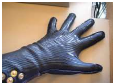
Fig. 8 - The sensorized glove considered to monitor the movements of the user's fingers.
