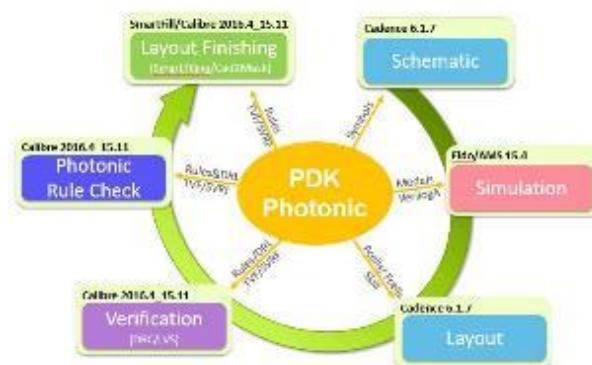
Figure 11: CEA-LETI photonic design flow
