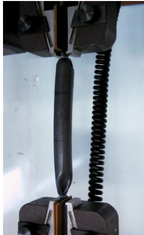
Figure 12. 3 Set-up of the tensile tests of the tubes filled with oil.
