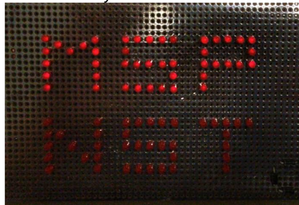
Fig. 3b: P(VDF-TrFE-CTFE) based piezo energy harvester with enough output power for driving 44 LEDs forming the MSP-letters.
