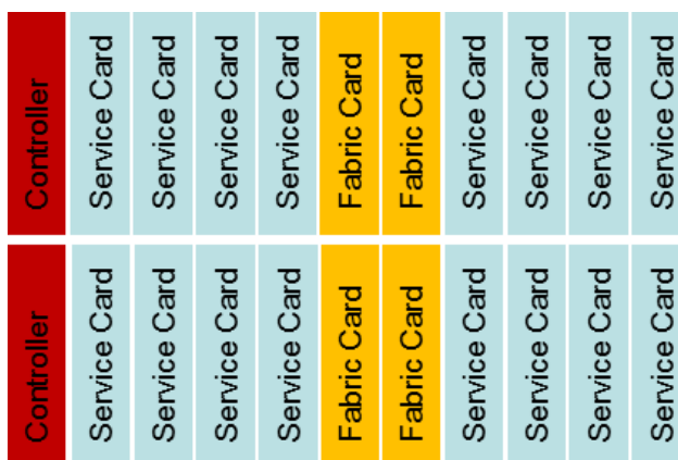
Figure 3-10: architecture of the DISCUS MPLS-TP core switch.
