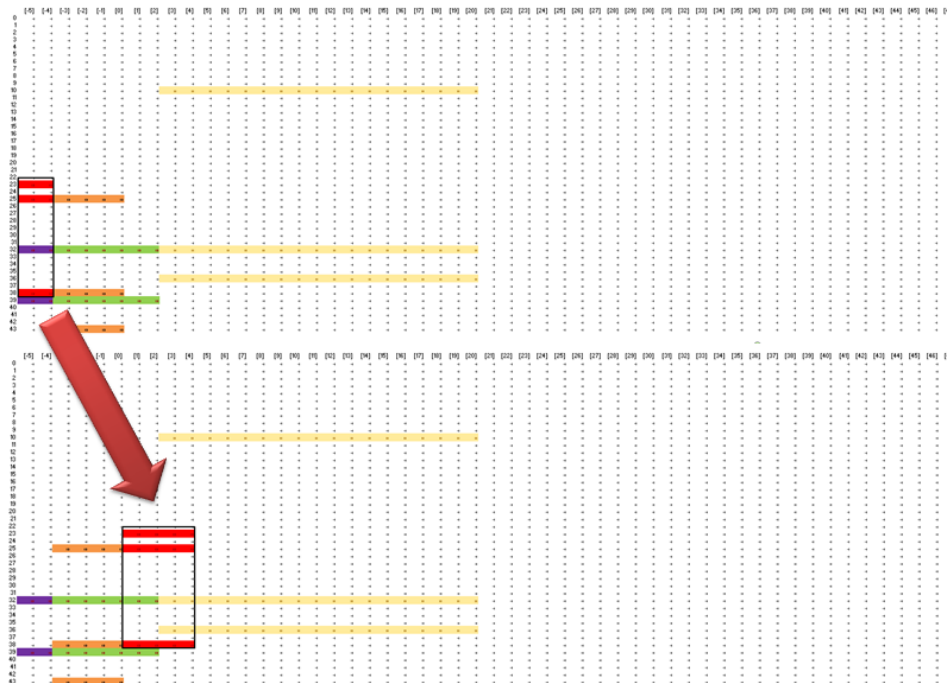
Figure 2-4: Reallocation of bandwidth for a particular channel.
