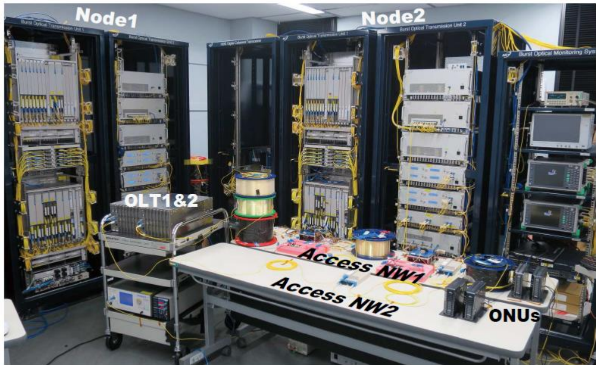
Fig. 6. Photo of the NICT experimental setup of an end-to-end network with optical packet/circuit switch nodes and extended-reach PON. (Courtesy of NICT)
