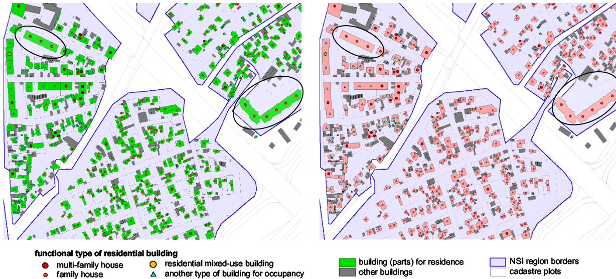
Figure 2-9: original buildings (now called “parts”, left) and generated “building blocks” ( right) due to dissolve operation
