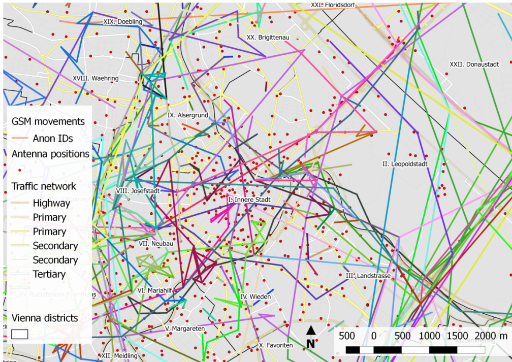
Figure 2: Data integration example: Visualisation of primary data of A1 GSM movement data derived from a generic binary log file converted to a GIS dataset showing a subset of 3000 anonymous IDs movements.
