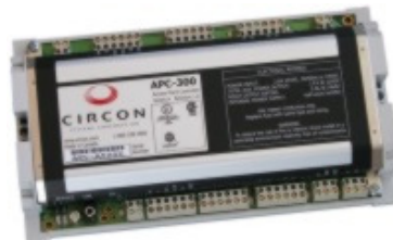
Figure 26: Elevator access control module 22
