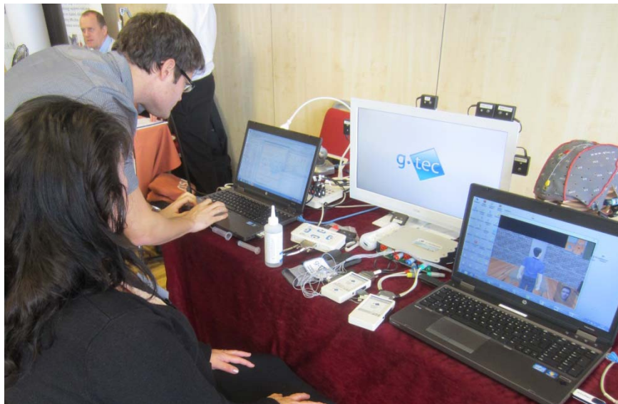
Figure 3: Final Prototype with input sensors and input screen (middle), BCI system (left computer) and Aml computer (right computer).
