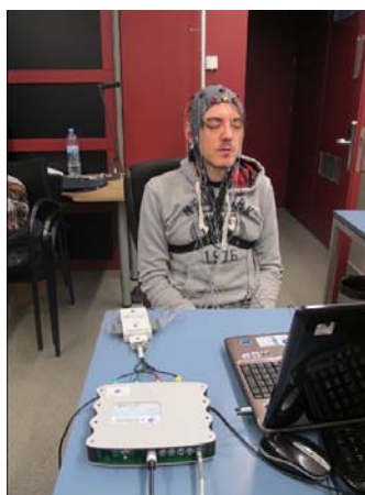
Figure 11: The experimental setup for cognitive stimulation using gUSBamp, Gammabox hardware by G.tec
